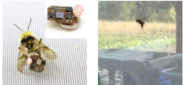
Figure 1: Living IoT platform on a bumblebee. (Left) Bee carrying our platform; (Right) Bee flying with our platform.
